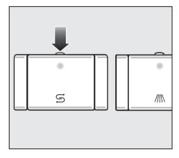
■ Press the button on the lid of the salt reservoir in the direction of the arrow until the flap springs open.
